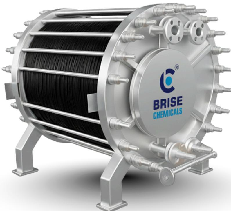
Brise Chemicals offers high-efficiency **bipolar alkaline hydrogen electrolyzers** that split high-purity Deionized water into hydrogen and oxygen using DC power. In our compact bipolar design, hydrogen forms at the **cathode** and oxygen at the **anode**, delivering higher efficiency and reduced internal losses. The system operates at **0-30** bar, producing pressurized hydrogen without the need for a separate compressor.
